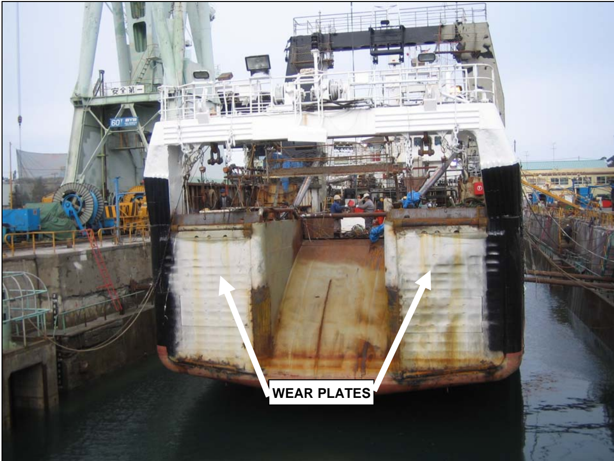
Figure 6. Wear plates fitted over stern of Alaska Ranger , shown in 2005. Stern ramp in the center allowed nets to be launched into the sea and then hauled on board with their catch.
